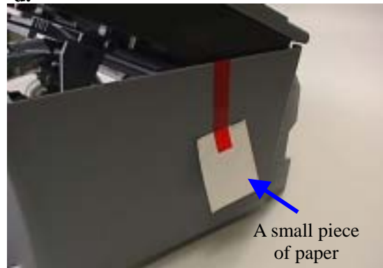
Figure 1-38 How to fix the Carriage
