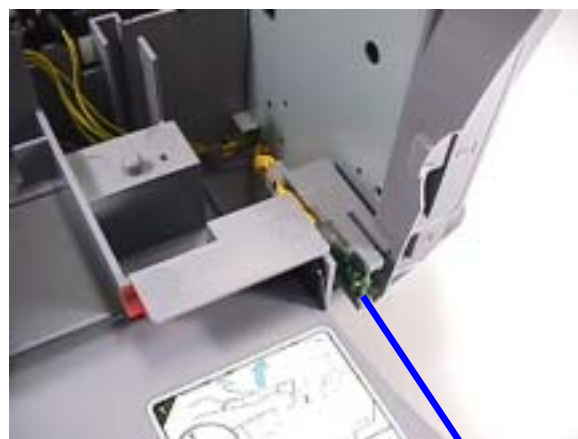
Figure 1-7 Cable Guide wiring
